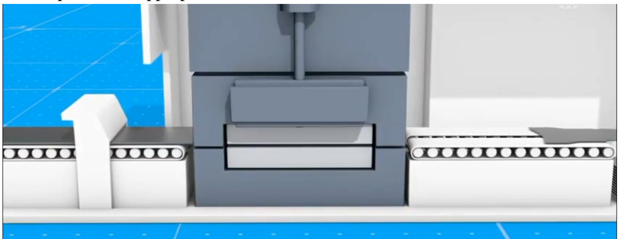
Fig.1. The hot forming process starts with blanking
