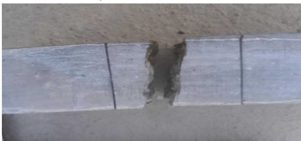
4-rasm. Materialning siniq yuzasida tabiiy ilashish mexanizmini amalda ko‘rsatish.
