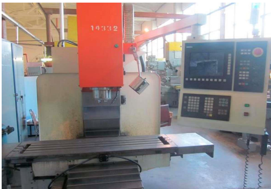
Figure 2.28. Vertical milling machine with CNC 6B52F3.
