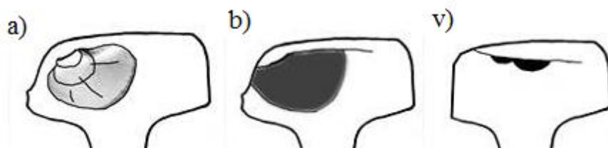
Fig. 2 Schematic representation of the rail defect [2].
