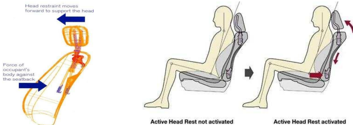
Figure 3 Working of Active Head Rest System
