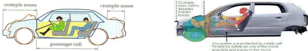
Figure 1 Crumple zone position
