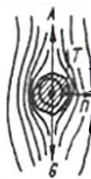
Fig.1. Forces acting on a particle in a viscous medium. A and friction force T.
