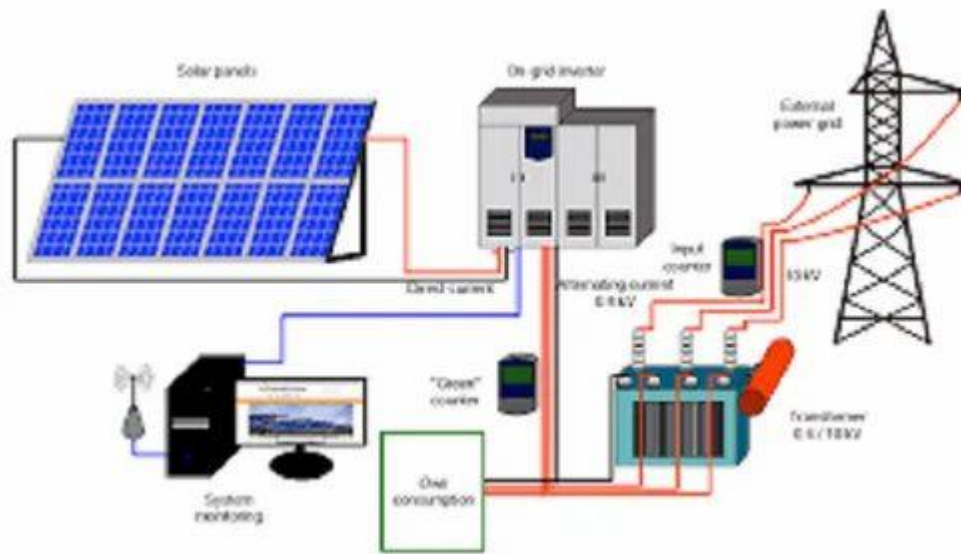
Figure 2. System design for solar projects
